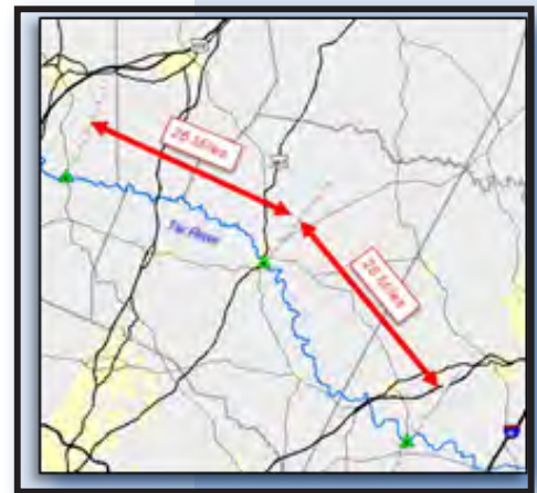
Typical Gage Distribution along Stream
