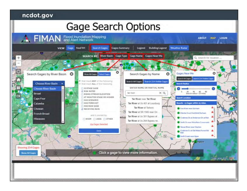
A specific stream or precipitation gage can be located by major river, gage type, gage name or using a geographic radius based on your approximate location.
