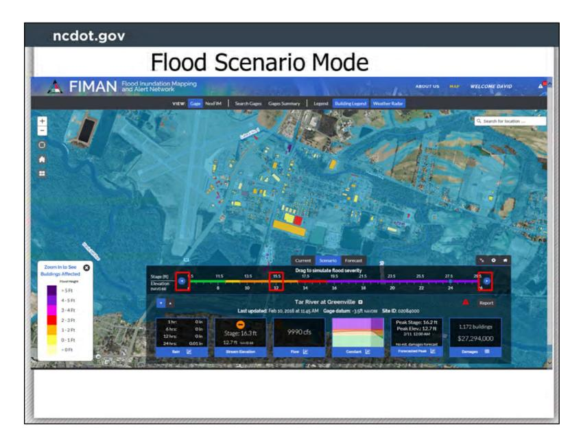
Flood extents and impacts for various flood levels can be visualized using the scenario tab on the dashboard. You can select different flood stages using the arrows at the left or right or by dragging the button on the stage graphic.
