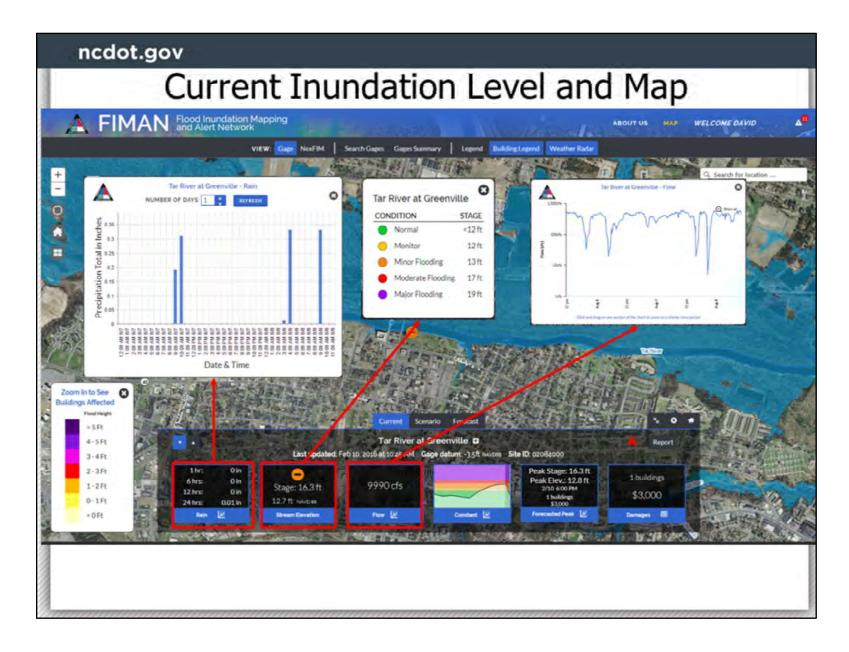
All items along the gage dashboard are interactive and dynamic. Clicking on the Rain window will bring up the rainfall hyetograph if available. The stream elevation window will show the gage specific flood risk rating stages and the flow tab has the hydrograph for the last 30 days.
