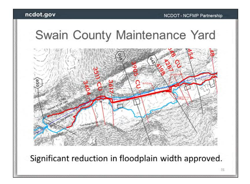
Additionally, the 100 year flow was able to be contained in a closed pipe system through the proposed building site significantly reducing the floodplain width, so the proposed building could be built outside the SFHA. Approved as a Type 2b MOA (Limited Detailed Study stream).
