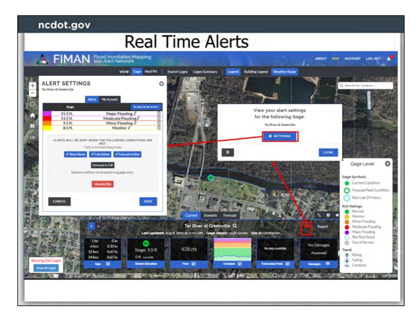
The alert tab allows users that have logged in to set up automated alerts and notifications based on a selected current or forecast flood level. Notified by text and email.
