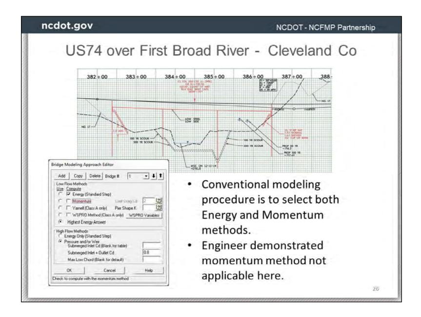
Conventional modeling caused increase in BFE which would have required a CLOMR. Good communication/documentation allowed qualification for approval as MOA Type 2d.
