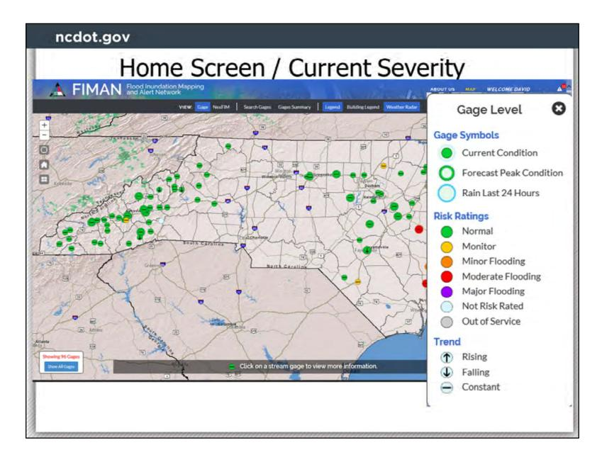
After you login the home screen will appear which includes gages color coded by flood risk severity. The inter ring color indicates current conditions and the center ring indicates forecast conditions. An outer halo indicates gages that have had rainfall in the last 24 hours. The flood stage trend of rising falling or constant are indicated by the arrows and hash mark in the center of the symbol.
